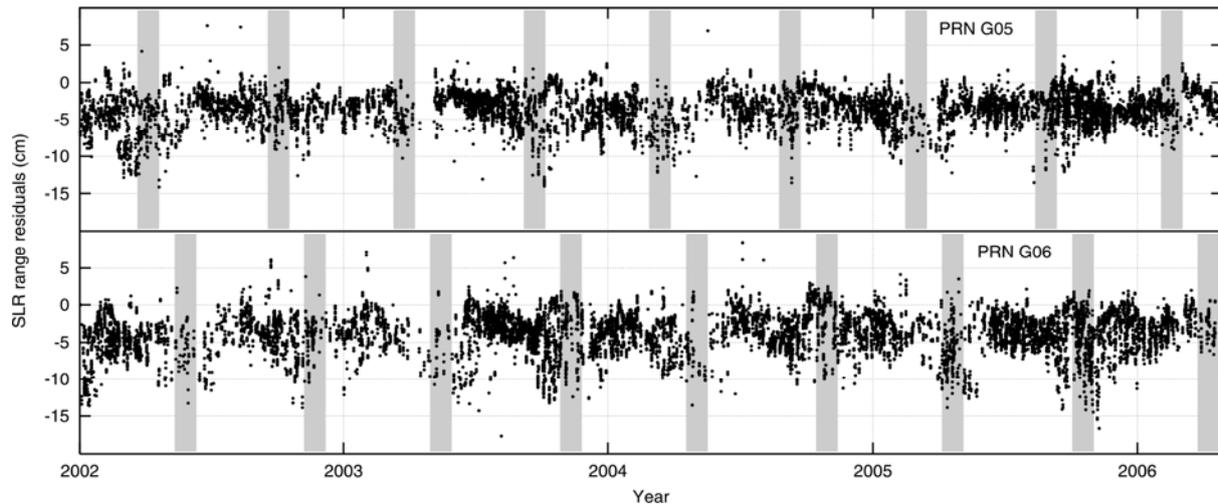
*Figure 1. SLR range residuals in cm for GPS satellites PRN G05 and G06, derived from CODE final orbits. The shaded areas indicate eclipse seasons*
