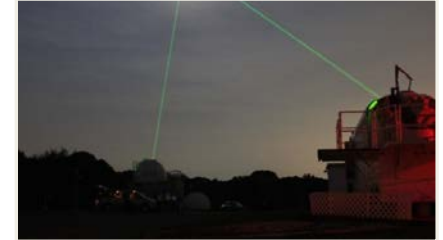
NGSLR & MOBLAS-7 simultaneously ranging at the Goddard Geophysical and Astronomical Observatory (GGAO)
